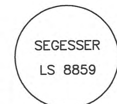
Typical Plastic Cap on set 5/8" Rebar
