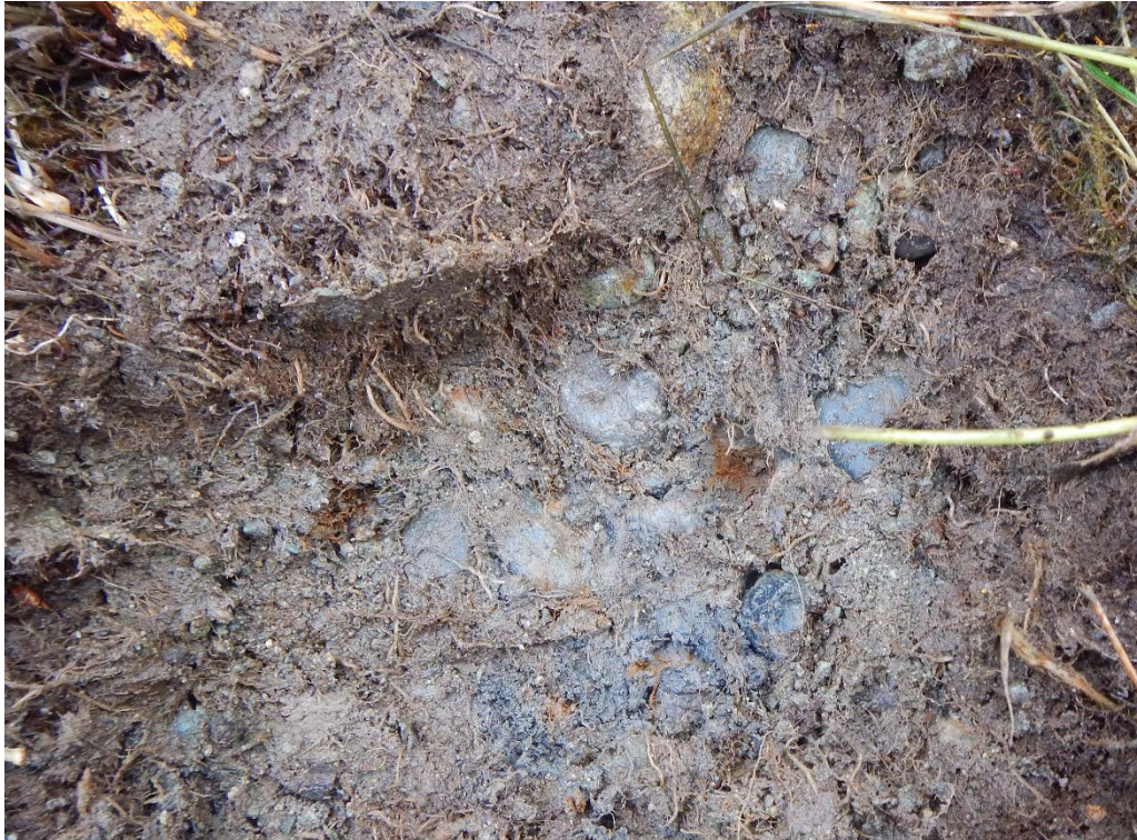
Picture 2. Presence of gleyed soils and iron deposits at TP 1.
