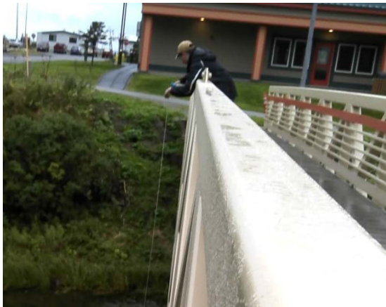
Photo 4-1. High School Student Measuring Transparency of the Water
